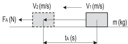
$$F_A = m \cdot \alpha = m \cdot \frac{V_2 - V_1}{t_A} \text{ (kgf)}$$
