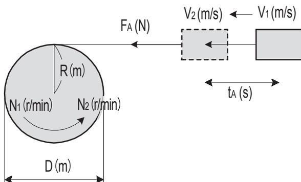
$$T_A = F_A \cdot R, \quad F_A = m \cdot \frac{V_2 - V_1}{t_A}$$
