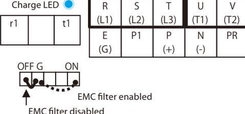
**Fig.2 200V class:HF4322-015, HF4322-022(15, 22kW)**
