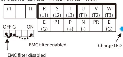
**Fig.4 400V class:HF4324-015, HF4324-022(15, 22kW)**
