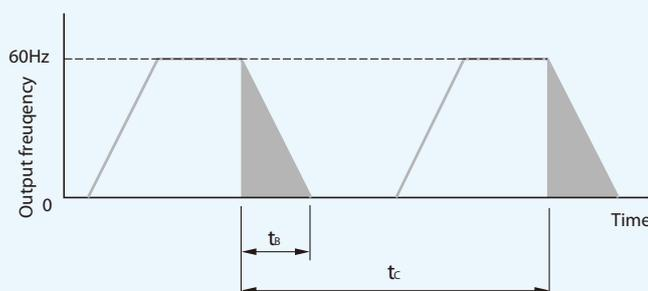
$$\text{Operating rate \%ED} = \frac{t_b}{t_c} \times 100$$
