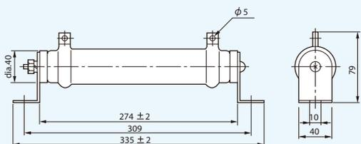
Note: When mounting the braking resistor, keep at least a 50mm clearance around the resistor.
