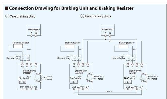
Note: 1. Connect a thermal relay to braking resistor and when operating, please cut the power supply of the inverter off.
