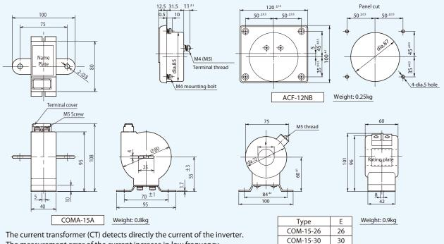
The measurement error of the current increase in low frequency.
